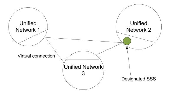
It can be observed in the diagram that Networks 1 and 3 connect through the Designates SSS installed in Network 2 that also share the same SSS with the rest.
